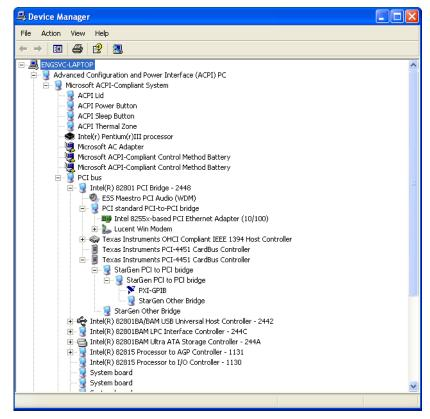
Figure 2-7. PXI Module Shown In Device Manager Tree
